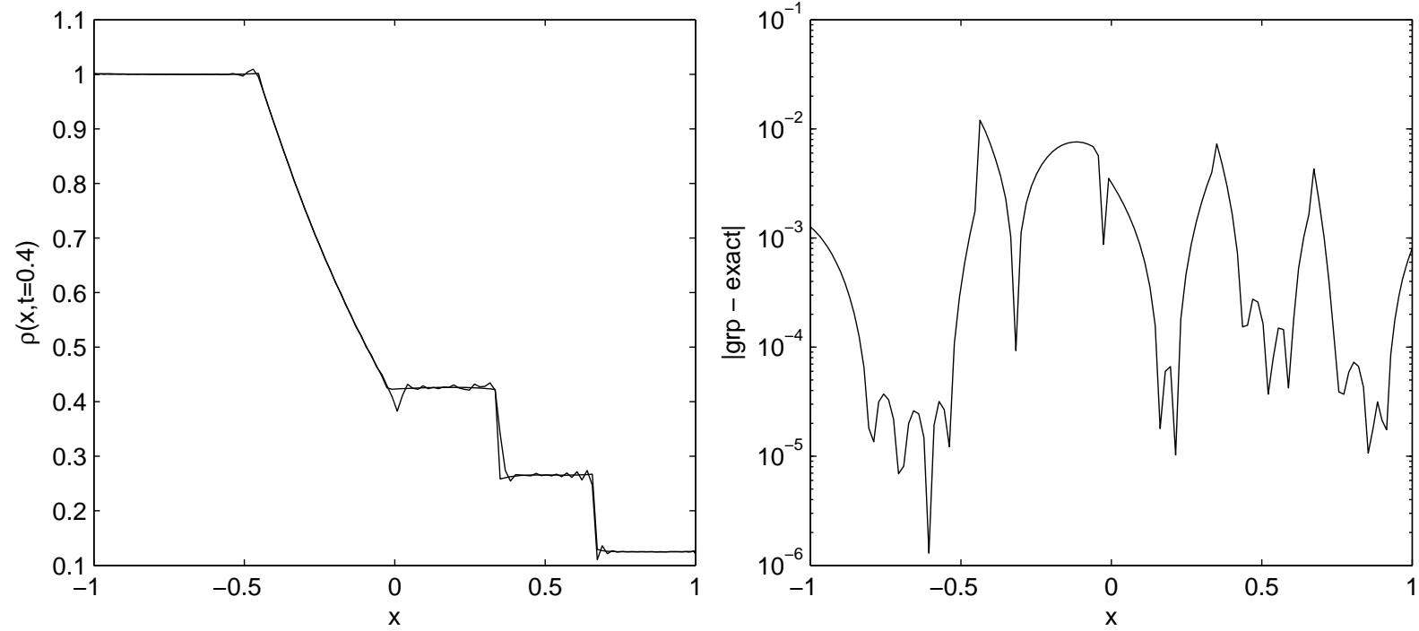
Chebyshev spectral viscosity and GRP postprocessed Euler density solution at time  $t = 0.4$ .
